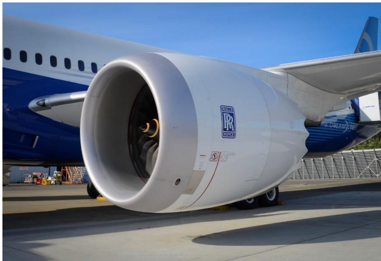
Figure 5. 2 Rolls Royce jet engine on Boeing 787. From Rolls Royce for aircraft. Retrieved from http://aircraft.sewaro.us/rolls-royce-engine-for-aircraft/ .
